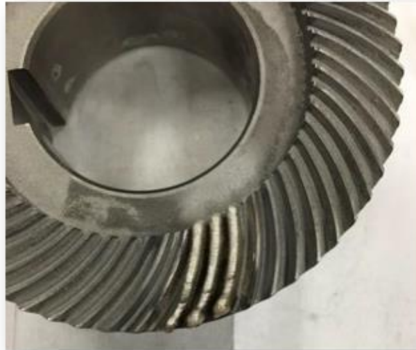
After repair with DED
