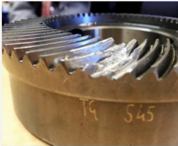
Broken gear teeth
